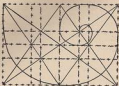
FIG. 100. SQUA. TWO DIVIDED INTO THREE EQUAL PARTS AND USING THE RHYTHMIC CURVE
