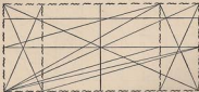
FIG. 135. ROOT FIVE WITH A ROOT FIVE AT EACH END WITH DIAGONALS AND PARALLEL LINES
